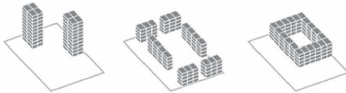
Fig. 1. Different types of buildings with the same number of dwellings, with different build-up and indicative housing density
